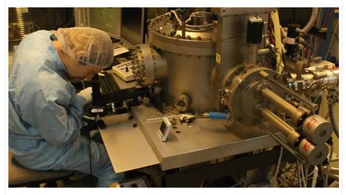
Optaglio holograms are created with e-beam lithography. This technology works with electron beam instead of a laser. The electron beam can be narrowed and broaden to create special effects while keeping reasonable effectivity.
